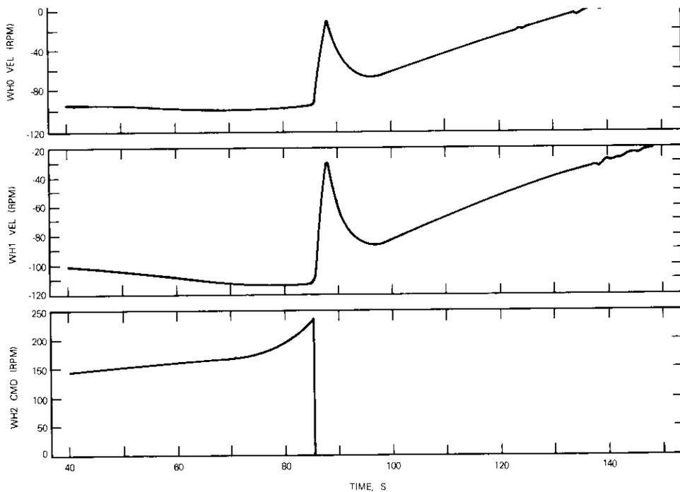
Figure 9. Wheel Failure with Three Reaction Wheels (sheet 2 of 3)
