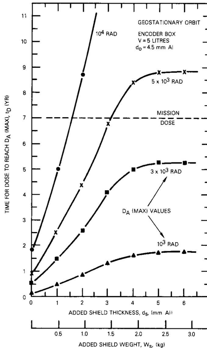
Figure 2. Survival of CMOS Circuits in a Particular Location of a Communications Satellite (from Reference 3)
