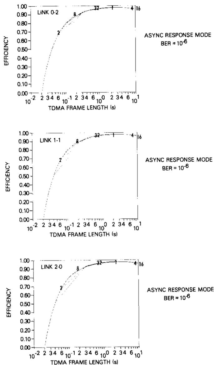
Figure 20. Net Throughput Efficiency for Piggybacked Acknowledgments With All Nodes Transmitting and a Preamble Plus Guard Time of 5 ms ( $BER = 10^{-6}$ ; curves represent different superframe sizes in K bytes)
