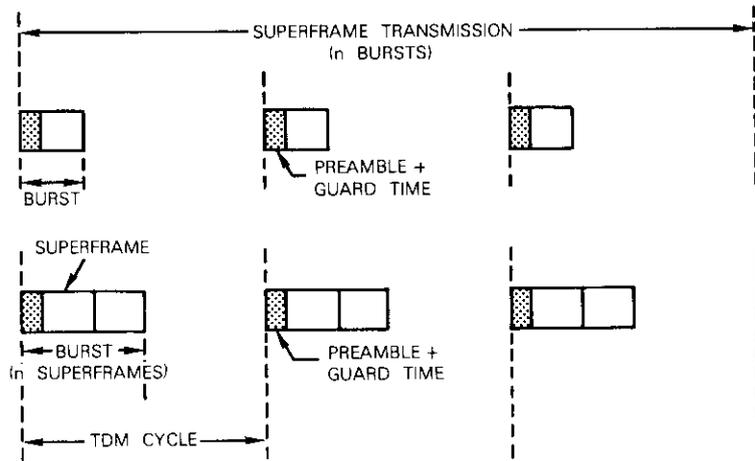
Figure 3. Illustration of the Case of Multiple Bursts per Superframe and the Case of Multiple Superframes per Burst
