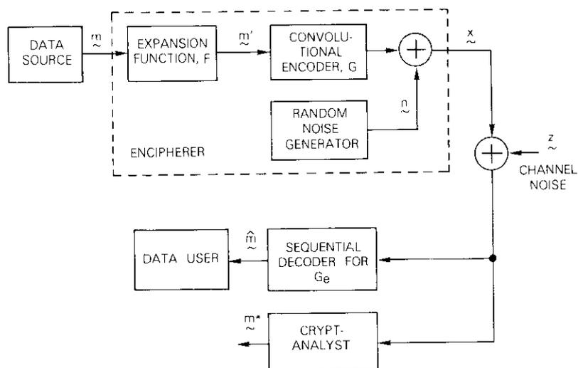
Figure 2. Block Diagram of the Proposed Cryptosystem
