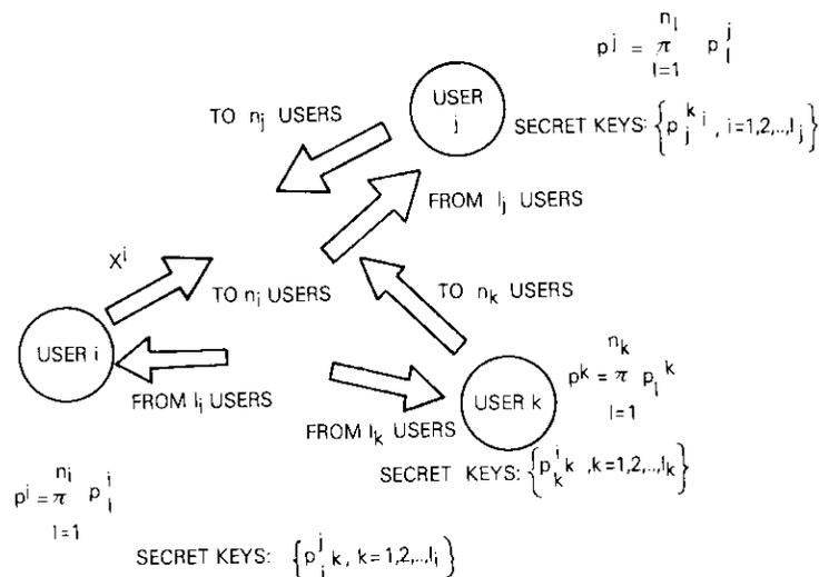
Figure 2. System Configuration of the Proposed Multiple-Destination Cryptosystem
