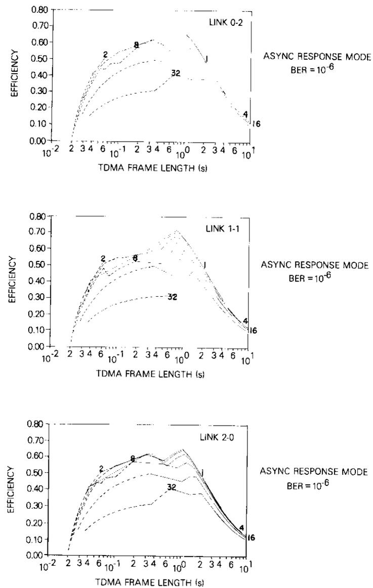
Figure 21. Net Throughput Efficiency for Piggybacked Acknowledgments With All Nodes Transmitting and a Preamble Plus Guard Time of 5 ms ( $BER = 10^{-8}$ ; curves represent different superframe sizes in K bytes)
