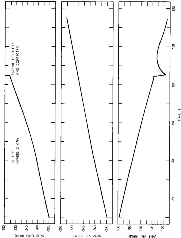
Figure 10. Wheel Failure with Four Reaction Wheels (Example 1) (sheet 3 of 3)
