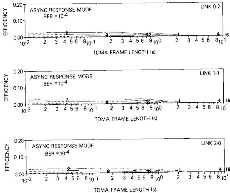
Figure 10. Net Throughput Efficiency for One-Way Data Flow and a Preamble Plus Guard Time of 50  $\mu$ s ( $BER = 10^{-4}$ ; curves represent different superframe sizes in K bytes)
