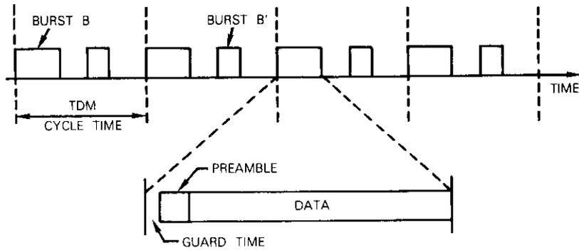
Figure 2. Representation of a TDM System With Bursts B Containing Link L and B' Containing Complementary Link L'
