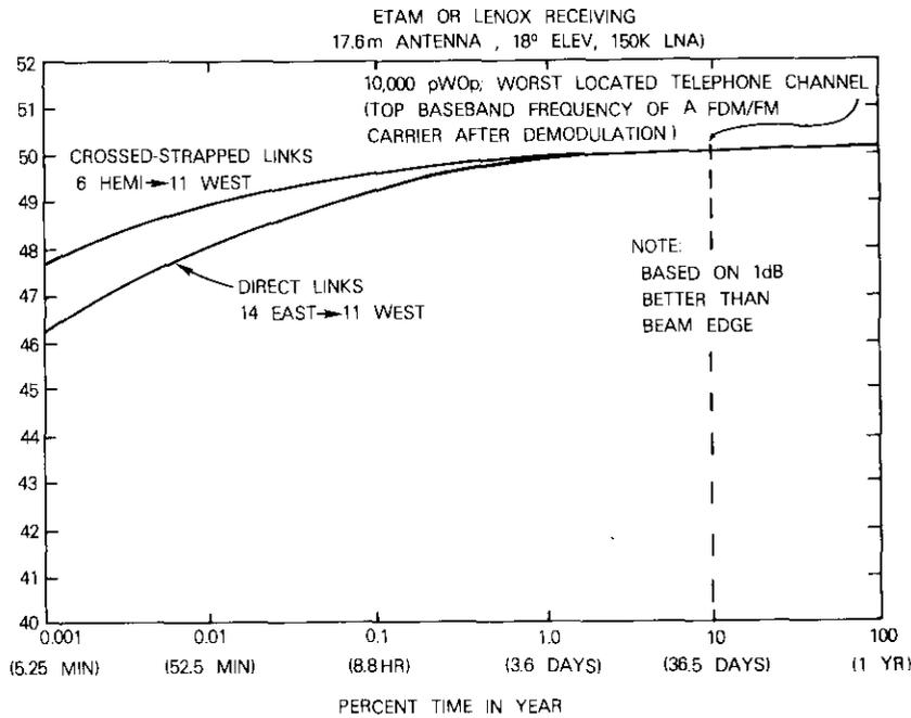
Figure 8. Telephone Channel Signal-to-Noise Ratio vs Time
