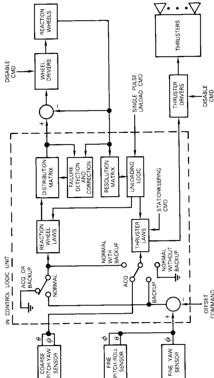
Figure 1. Simplified Block Diagram of the Control System
