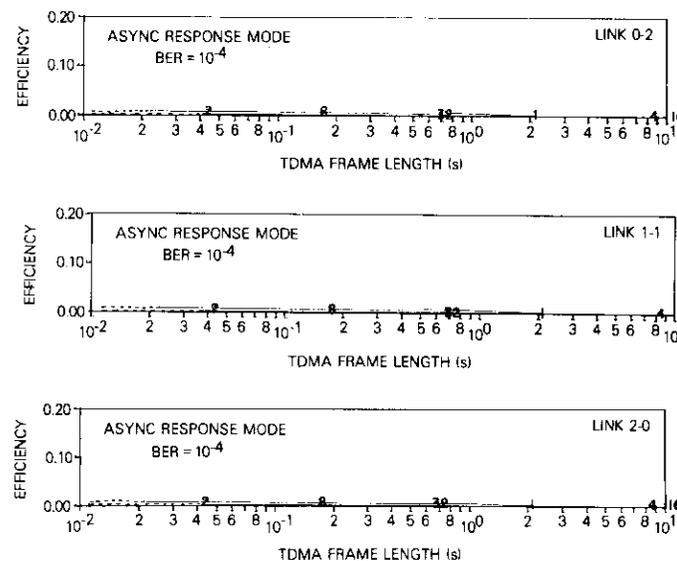
Figure 16. Net Throughput Efficiency for Piggybacked Acknowledgments With All Nodes Transmitting and a Preamble Plus Guard Time of 50  $\mu$ s ( $BER = 10^{-4}$ ; curves represent different superframe sizes in K bytes)
