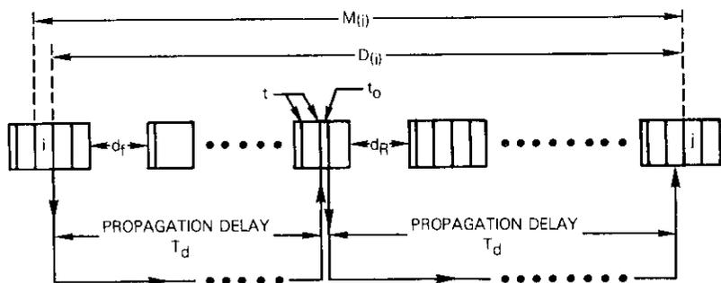
Figure 8. Illustration of Effective Propagation Delay  $D(i)$  in a TDM System in the Case of Multiple Superframe per Burst Operation and One-Way Data Flow
