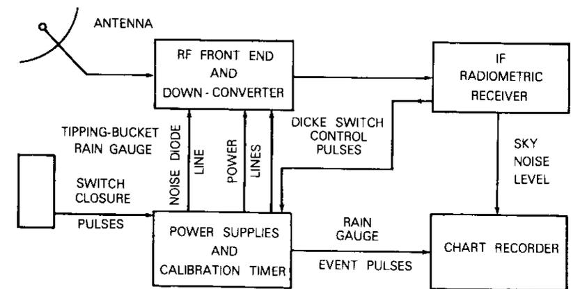
Figure 2. Block Diagram of Radiometric Receive Terminal
