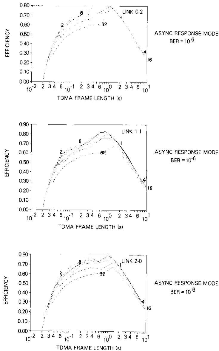
Figure 14. Net Throughput Efficiency for One-Way Data Flow and a Preamble Plus Guard Time of  $5 \text{ms}$  ( $\text{BER} = 10^{-6}$ ; curves represent different superframe sizes in K bytes)
