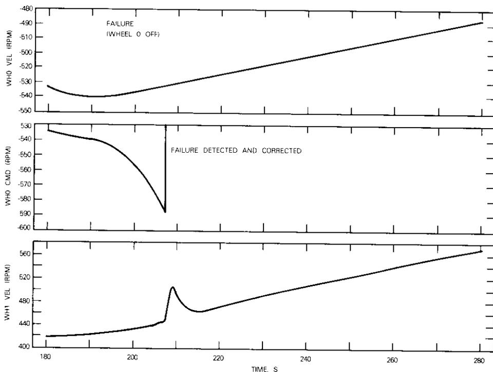
Figure 11. Wheel Failure with Four Reaction Wheels (Example 2)
