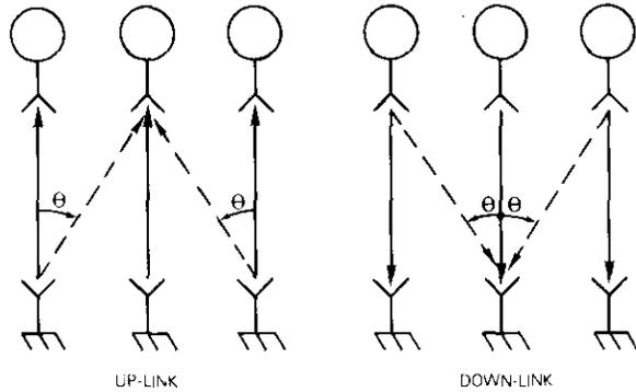
Figure 6a. Two Interfering Sources at Equal Angles
