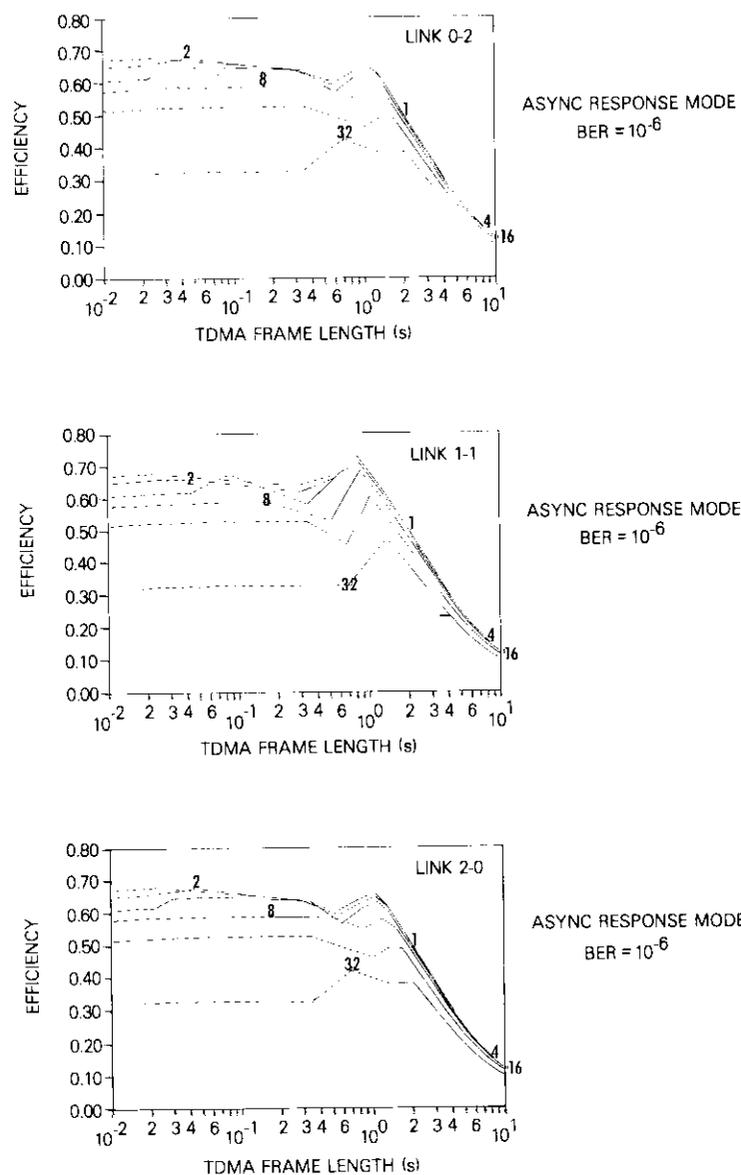
Figure 17. Net Throughput Efficiency for Piggybacked Acknowledgments With All Nodes Transmitting and a Preamble Plus Guard Time of 50  $\mu$ s ( $BER = 10^{-6}$ ; curves represent different superframe sizes in K bytes)
