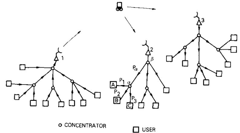
Figure 4. A Typical Architecture of Digital Communications Networks with Levels of Hierarchy
