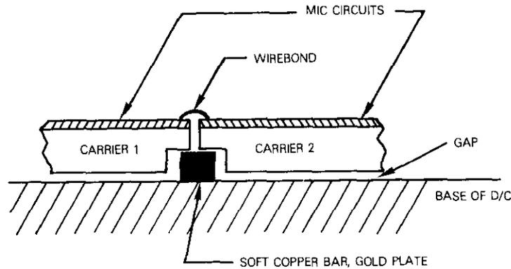
Figure 6. Details of MIC Interconnection Technology
