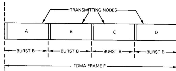
Figure 9. Representation of Example Satellite TDMA System With Four Nodes
