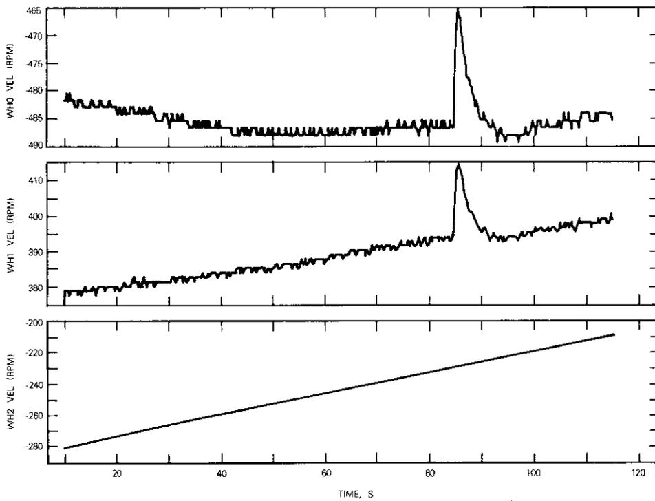
Figure 10. Wheel Failure with Four Reaction Wheels (Example 1)
