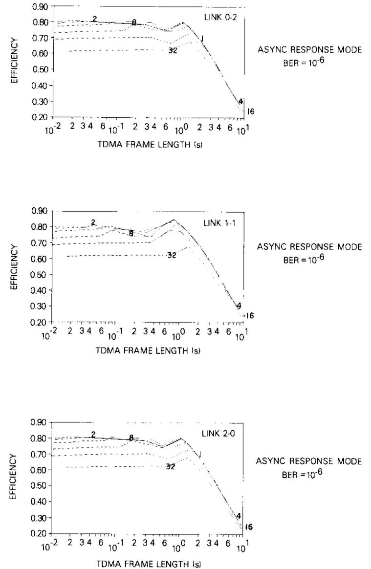
Figure 11. Net Throughput Efficiency for One-Way Data Flow and a Preamble Plus Guard Time of 50  $\mu$ s ( $BER = 10^{-6}$ ; curves represent different superframe sizes in K bytes)
