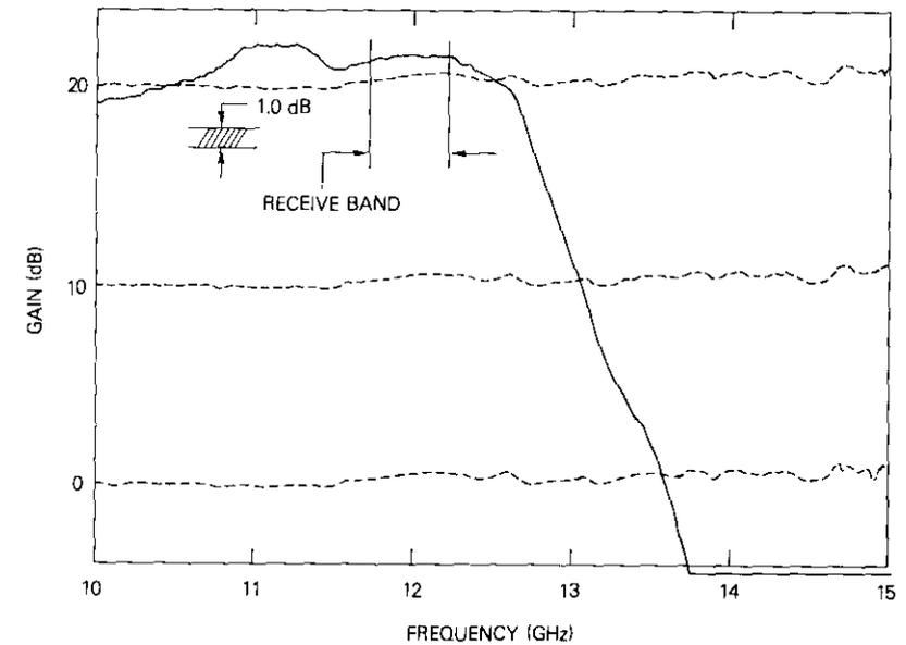
Figure 11. Wideband Measured Response of a 3-Stage Low-Noise Amplifier
