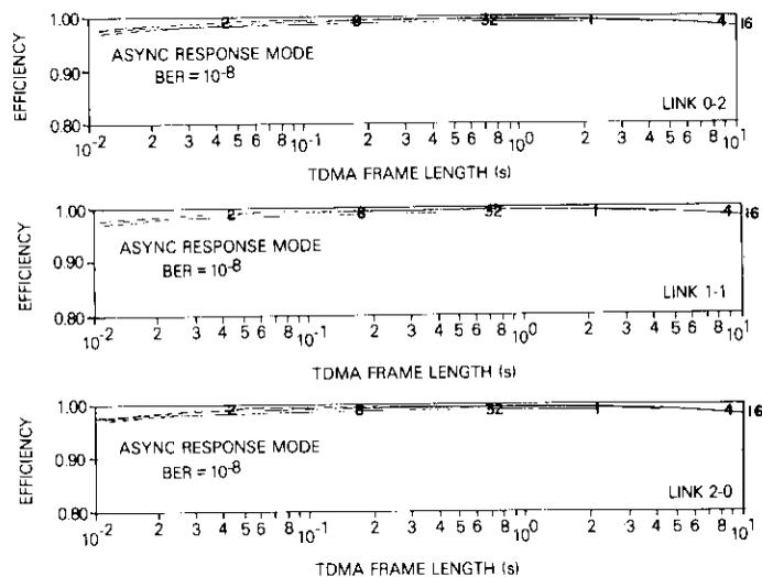
Figure 12. Net Throughput Efficiency for One-Way Data Flow and a Preamble Plus Guard Time of  $50 \mu\text{s}$  ( $\text{BER} = 10^{-8}$ ; curves represent different superframe sizes in K bytes)
