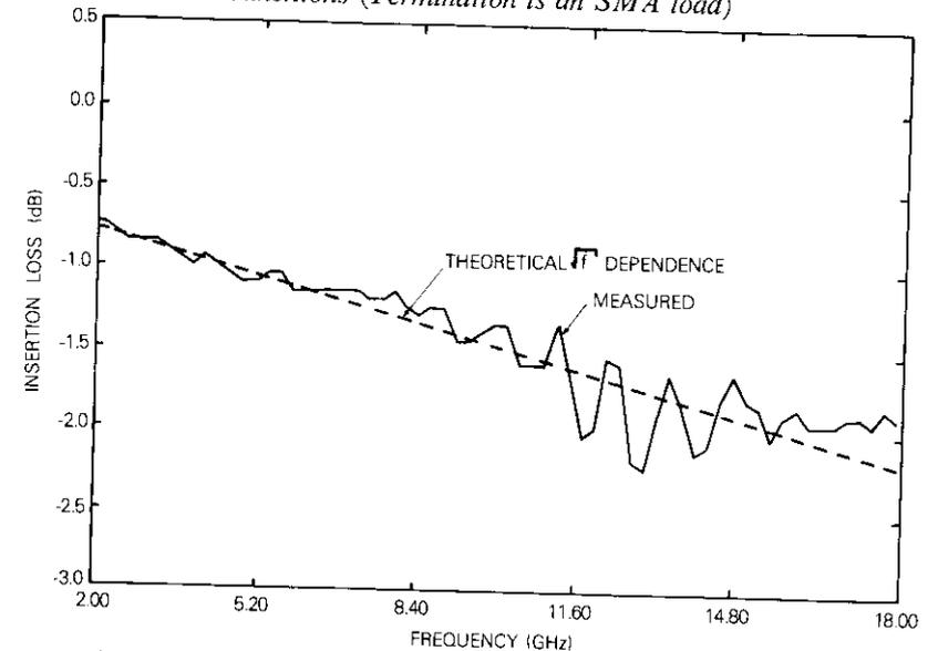
Figure 5. Measured Insertion Loss of a 5.08-cm CPW Line
