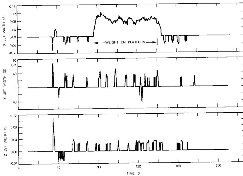
Figure 8. Stationkeeping by Applying a Weight on the Platform (thruster control) (sheet 2 of 3)
