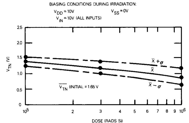
a. THRESHOLD VOLTAGE OF N-CHANNEL DEVICES,  $V_{TN}$  (INCLUDES ALL THREE LEVELS OF INTEGRATION; SOLID LINE INDICATES MEAN VALUE AND DASHED LINES INDICATE ONE STANDARD DEVIATION)
