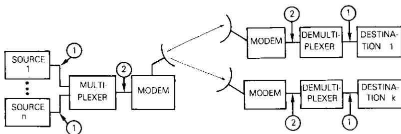
Figure 1. A Typical Broadcast Network and Two Commonly Used Approaches to Provide Communications Security
