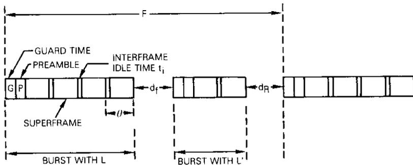
Figure 6. Representation of TDM System Case of Multiple Superframes per Burst Operation and Burst Structure
