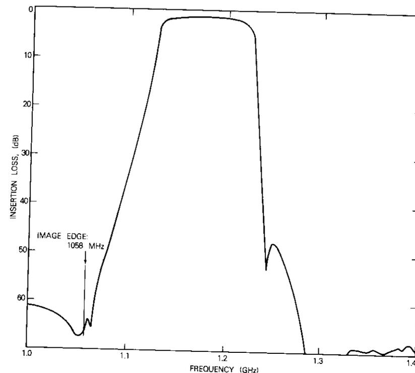
Figure 17. Measured Insertion Loss of IF Filter with  $N = 7$ ,
