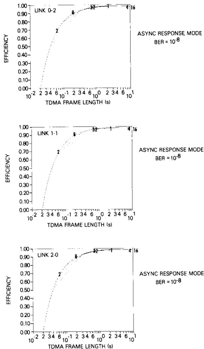
Figure 15. Net Throughput Efficiency for One-Way Data Flow and a Preamble Plus Guard Time of 5 ms ( $BER = 10^{-8}$ ; curves represent different superframe sizes in K bytes)
