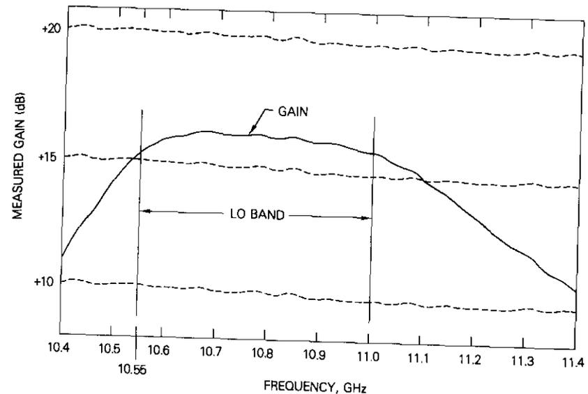
Figure 7. Measured Gain of FET LO Amplifier
