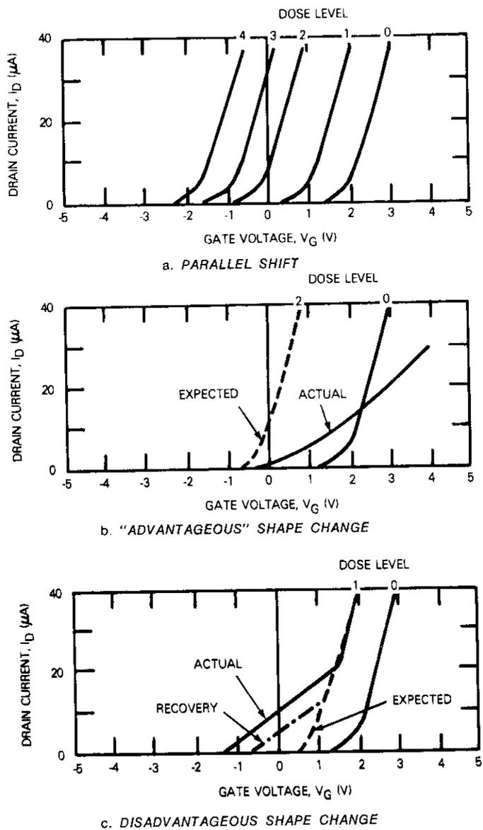
Figure 1. Effect of Irradiation on the Characteristics of an n-Channel MOS FET. The numbers representing dosage levels are only indicators; the actual dose level depends on many parameters (from Reference 3).
