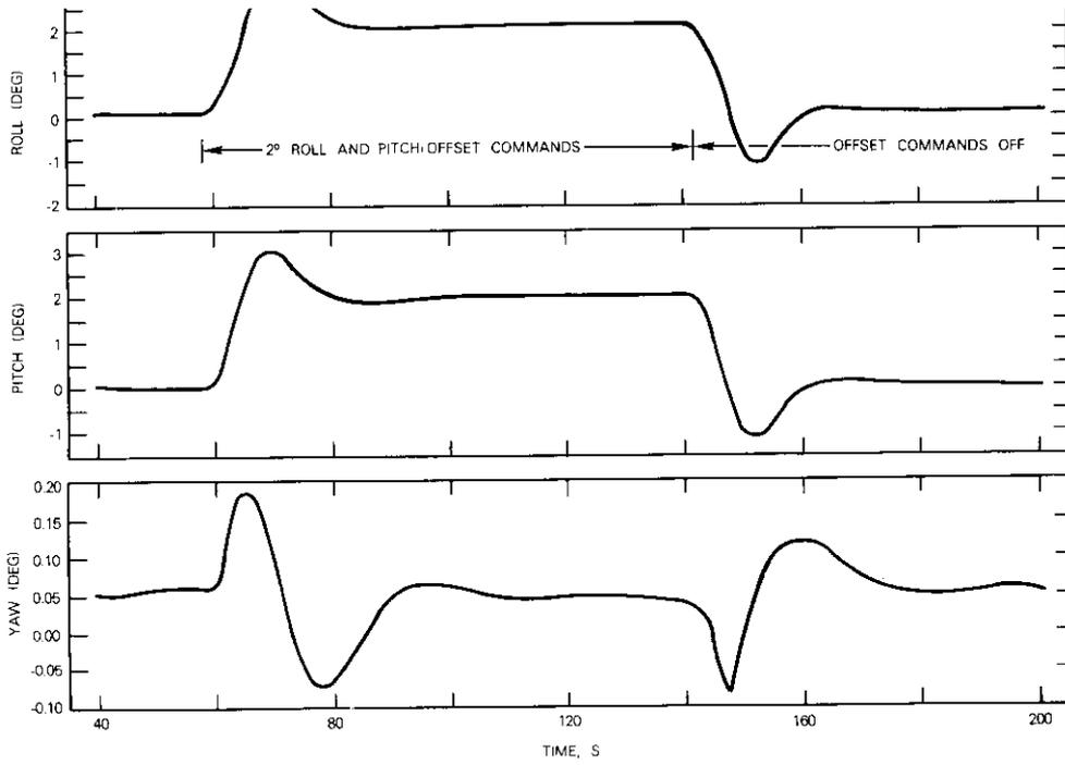
Figure 5. *Transient Response for Four Reaction Wheels*
