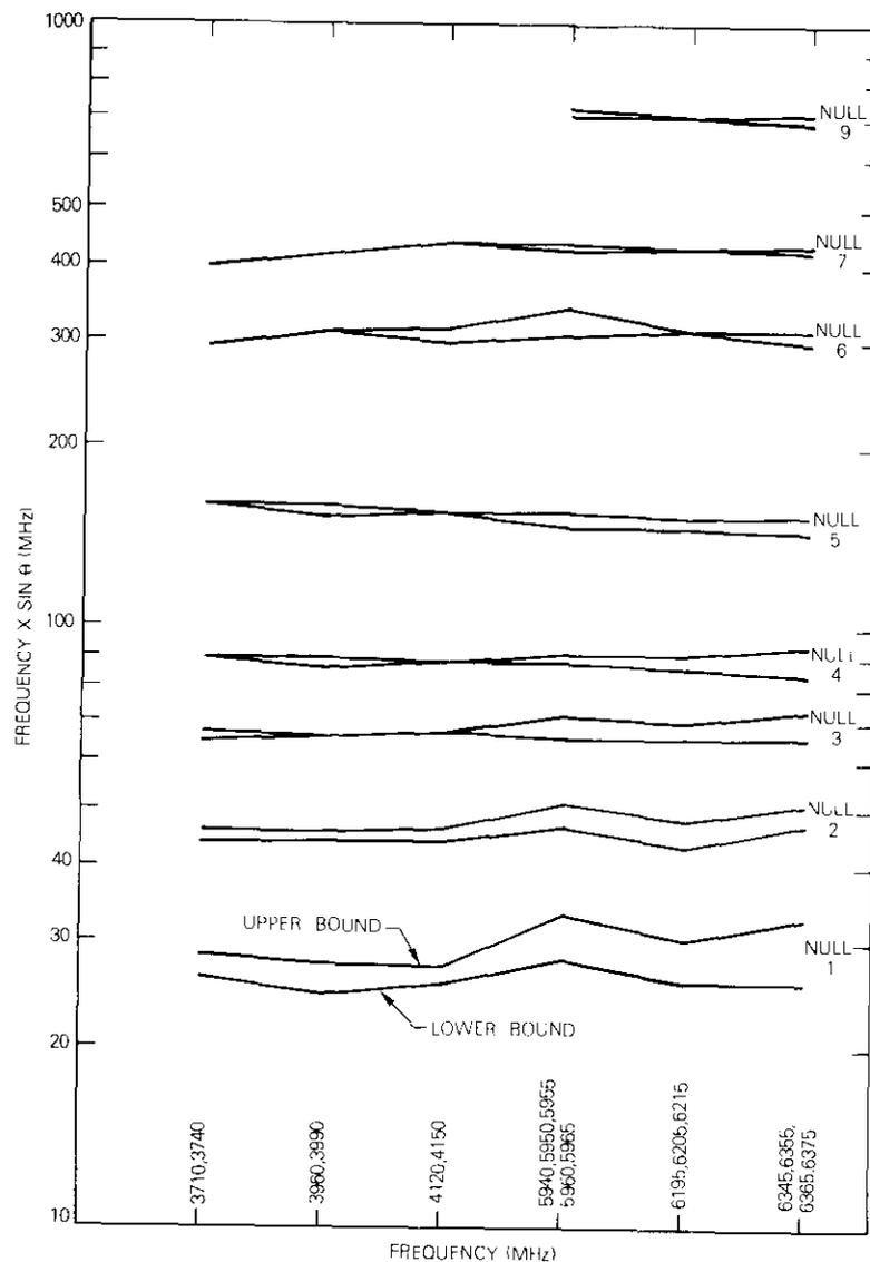
Figure 9. Freq-Sin  $\theta$  Product for Selected Nulls at Frequencies Across the Up- and Down-Bands
