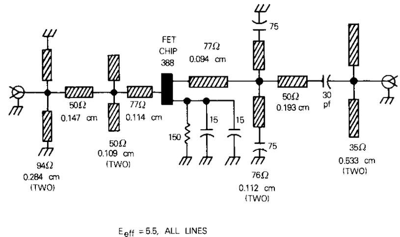
Figure 7. Equivalent Circuit for 1-Stage CPW FET Amplifier
