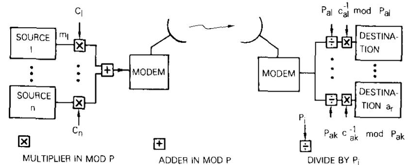
Figure 5. The Implementation of the Proposed Multiple-Destination Cryptosystem for Broadcast Networks
