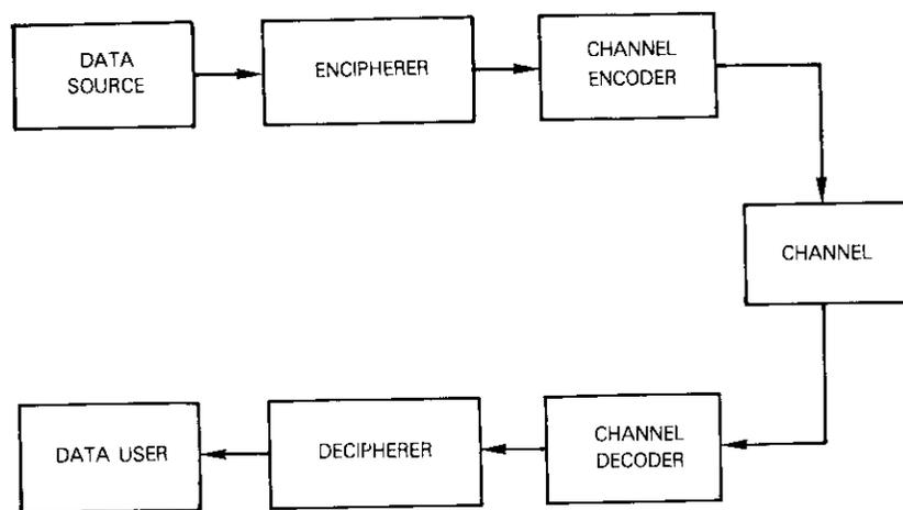
Figure 1. Block Diagram of a Typical System For Reliable and Secure Communications
