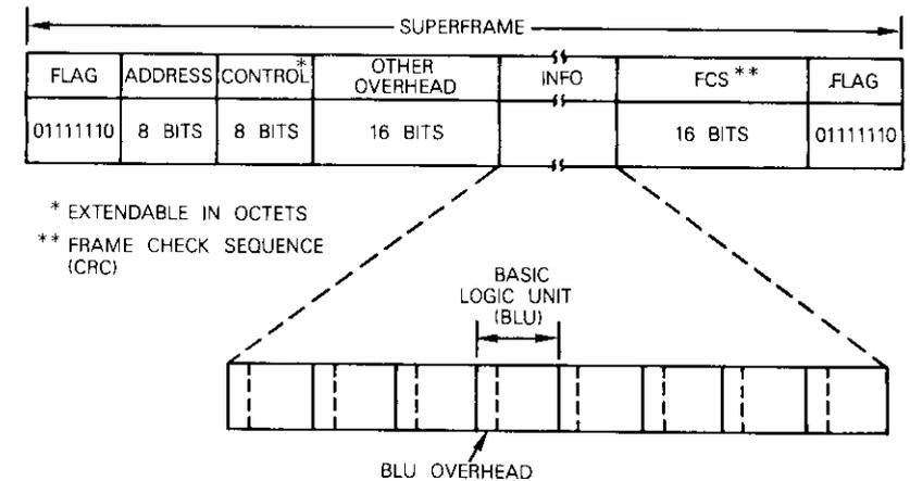
Figure 1. Superframe Format and BLU Structure (Basic logic units may all be for the same destination or for different destinations.)
