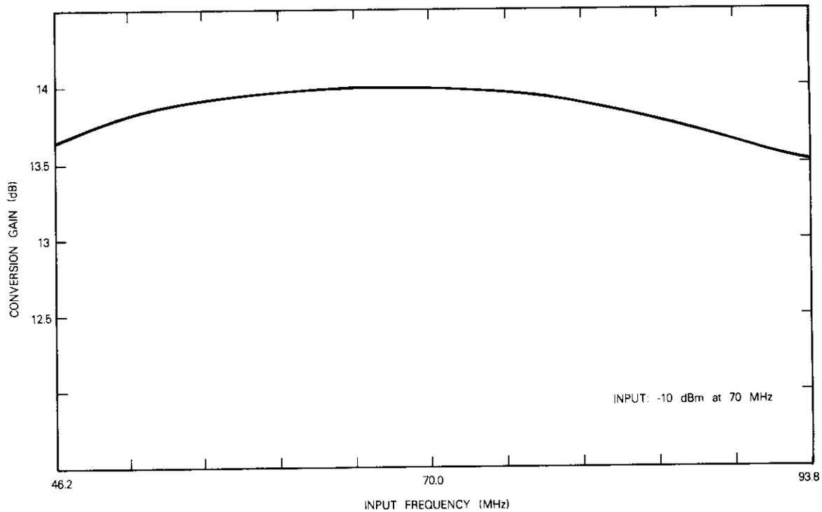
Figure 29. Measured Up-Converter Conversion Gain vs Input Frequency with an Output Frequency of 14 GHz (Second LO is fixed.)
