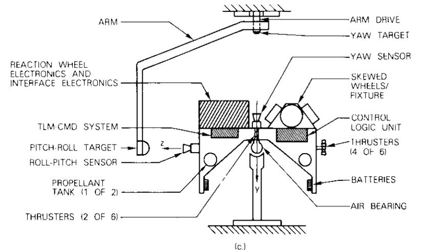
Figure 3. Control System on Test Facility
