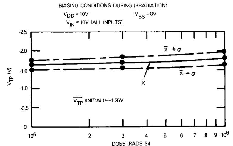
b. THRESHOLD VOLTAGE OF P-CHANNEL DEVICES,  $V_{TP}$  (INCLUDES ALL THREE LEVELS OF INTEGRATION; SOLID LINE INDICATES MEAN VALUE AND DASHED LINES INDICATE ONE STANDARD DEVIATION)
