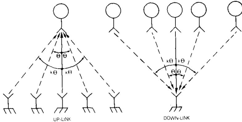
Figure 6b. Two Interfering Sources at Angle  $\theta$  and Two at  $k\theta$
