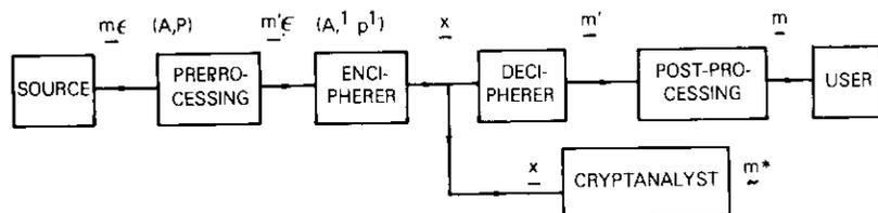
Figure 1. A Cryptosystem Using A Message Preprocessing Scheme to Reduce Message Pseudoredundancy and to Improve Security
