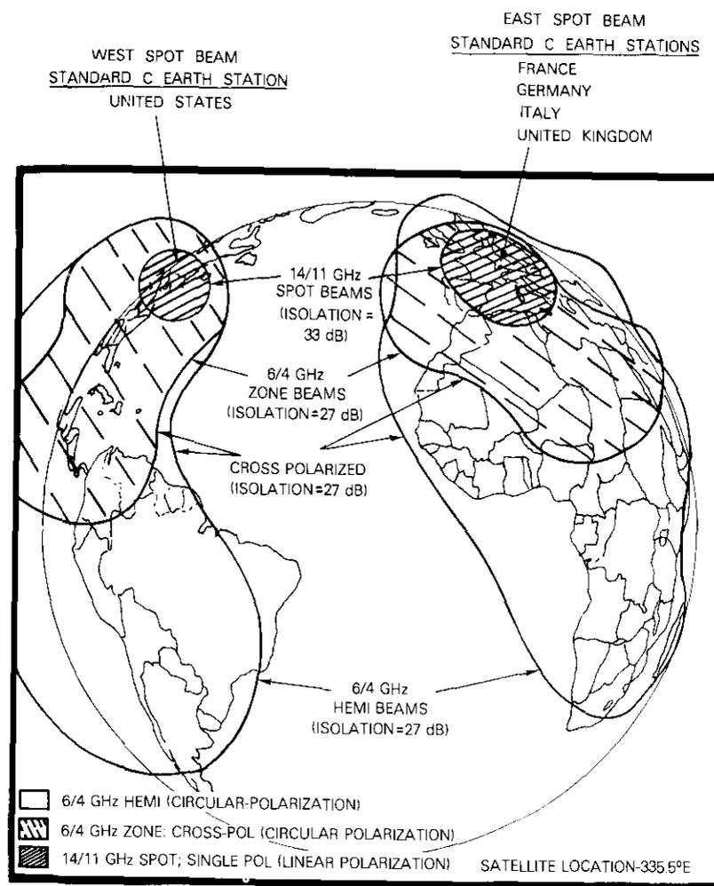
Figure 1. INTELSAT V Atlantic Satellite Transmit Capabilities for Standard C Earth Stations, Primary Satellite (14/11-GHz spot beams are steerable and may be moved to meet traffic requirements)
