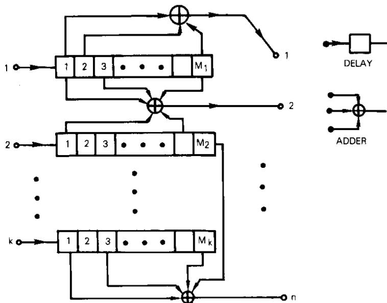
Figure 3.  $k$ -Input,  $n$ -Output Feed Forward Linear Sequential Circuit (FFLSC)
