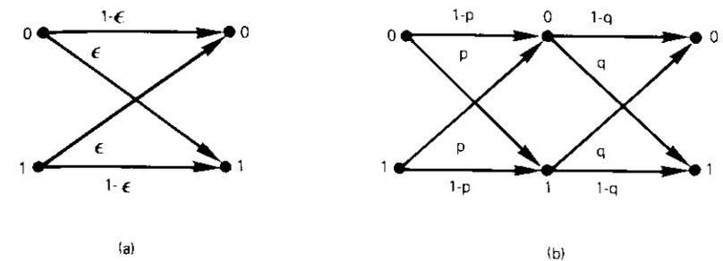
Figure 4(a) Binary Symmetric Channel with Crossover Probability  $\epsilon$
