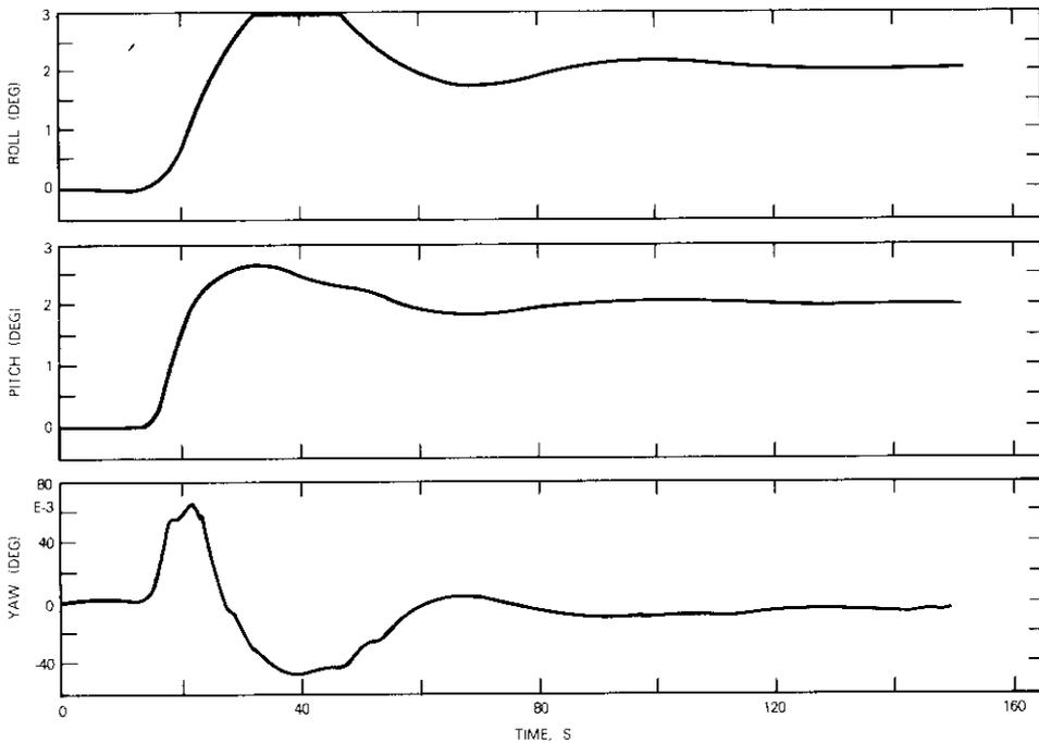
Figure 6. *Transient Response with Uncorrected Failure of Wheel 0 (offset commands)*
