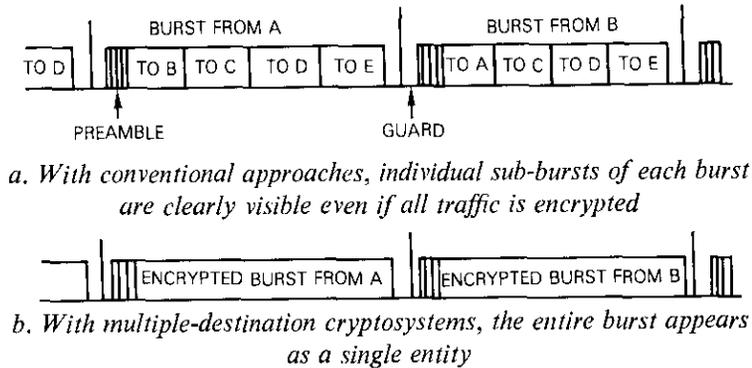
Figure 3. Typical TDMA Formats
