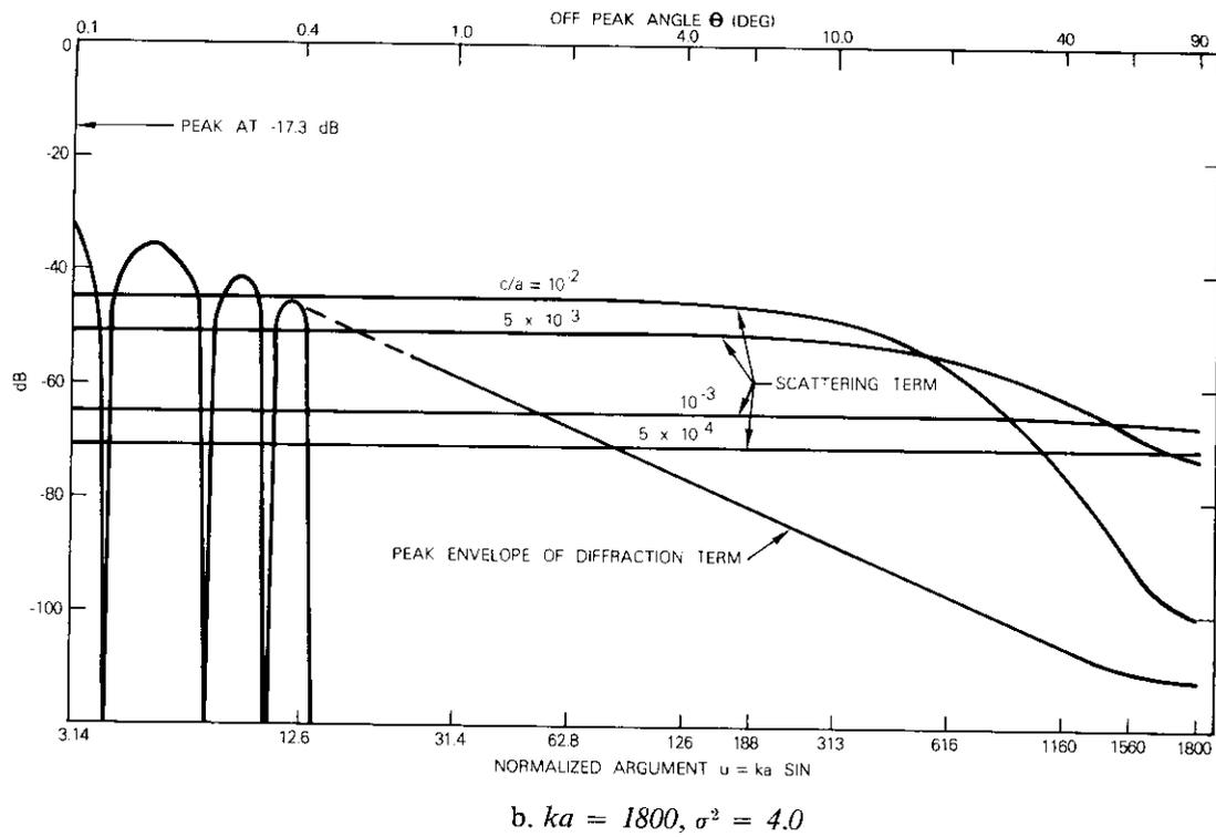
Figure 3. Diffraction and Scattering Terms of  $E\{gg^*\}$  vs Angle
