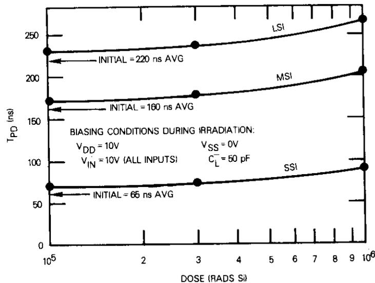
d. PROPAGATION DELAY,  $T_{PD}$ , FOR THREE LEVELS OF INTEGRATION
