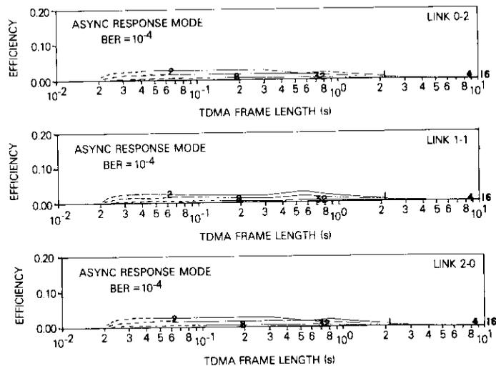
Figure 13. Net Throughput Efficiency for One-Way Data Flow and a Preamble Plus Guard Time of  $5 \text{ms}$  ( $\text{BER} = 10^{-4}$ ; curves represent different superframe sizes in K bytes)
