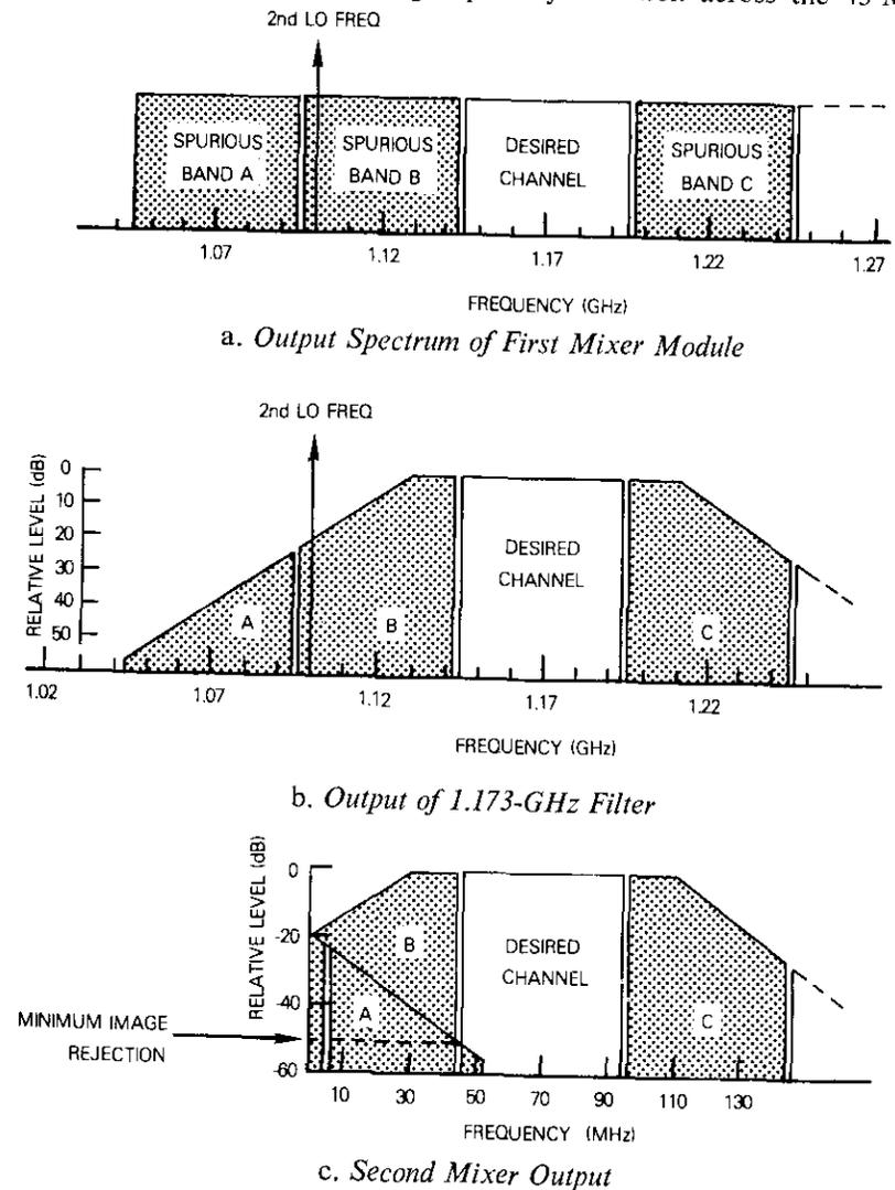
Figure 4. Frequency Plan of Down-Converter
