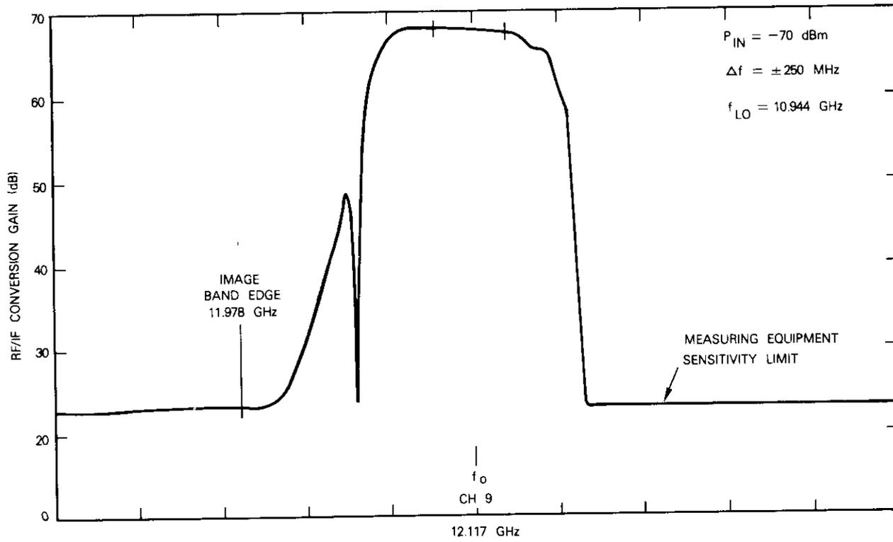
Figure 19. Down-Converter Conversion Gain vs Input Frequency (LO Chosen for Channel 9)
