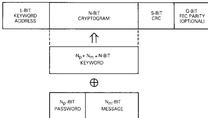
Figure 1. Data Format in Forward Link
