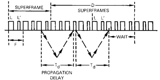
Figure 5. Representation of TDM System Case of Multiple Bursts per Superframe Operation With Short Acknowledgments
