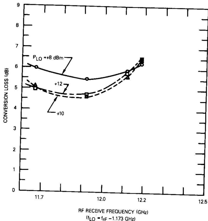
Figure 14. Measured MIC Mixer Performance
