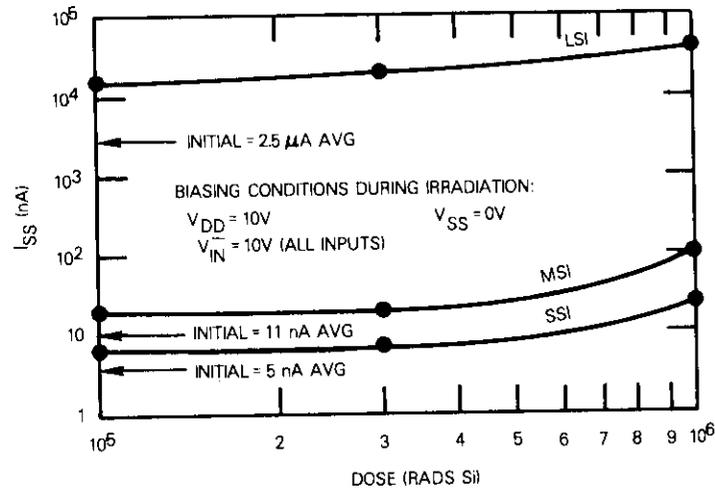
c. QUIESCENT CURRENT,  $I_{SS}$ , FOR THREE LEVELS OF INTEGRATION
