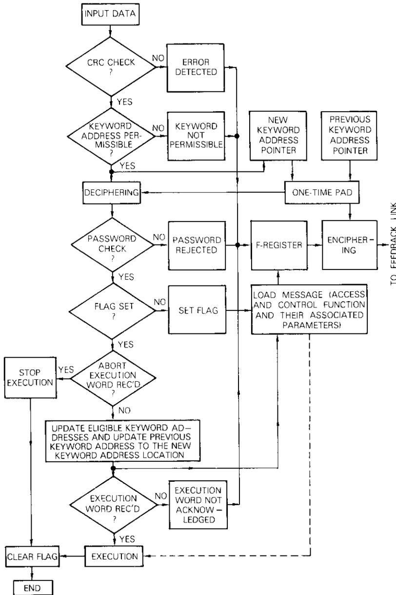
Figure 4. Flow Chart for the Recipient's Authentication Subsystem
