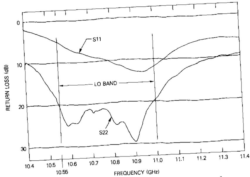
Figure 9. Return Losses Measured at Input and Output of FET LO Amplifier
