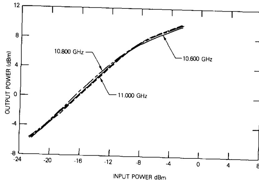
Figure 8. Saturation Characteristics of FET LO Amplifier
