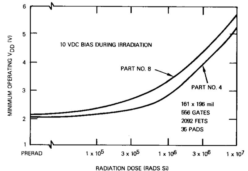
Figure 4. *Minimum Operating Voltage of a Multiplexer Control LSI Circuit (curves represent minimum and maximum shifts exhibited by six test chips) (from Reference 10)*
