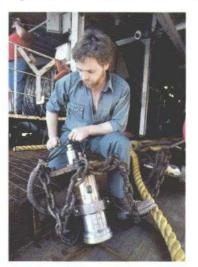
Bottom Left, Vetter crewman with one of the a pressure guns used to generate underwater sho wave, a vital part of seismic work. Below Right Small section of seismic vessel streamer cut op to reveal hydrophone.
