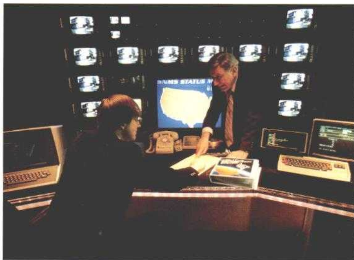
Above, In the Skypath Room at NBC-New York, Central control and monitoring of the Satellite Network Management System (SNMS) for the Comsat General/NBC Distribution System takes place here and in a similar room at NBC-Burbank. The most critical job of the satellite system is the switching function—telling the electronic traffic where to go. Skypath computers are loaded daily with switching information for all of the 181 earth stations in the system. Shown are NBC engineers Stev Asay, left, and Robert J. Butler, Chief Engineer, Satellite Network. Left, Distribution of "The Tonight Show Starring Johnny Carson" to over 200 NBC-affiliated stations starts at this video-feed machine at NBC-Burbank. Broadcast engineer John Griffin operates machine.
