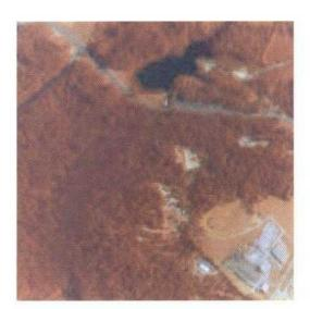
Magnified portions of a multispectral image of an airfield which has been compressed at 40:1 using spectral compression in conjunction with discrete cosine transform processing. The three-band composite images of the original (LEFT) and compressed/decompressed (NGUT) images are virtually indistinguishable.
