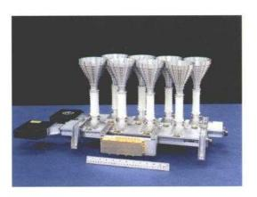
The high polarization purity of the elements in the X-band array makes it suitable for dualpolarization applications.
