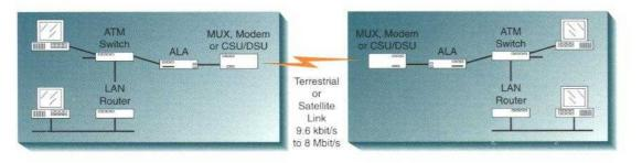
LEFT: The ATM Link Accelerator (ALA) interconnects ATM switches over satellite and wireless links at up to 8 Mbit/s. It offers adaptive coding, data compression, and congestion control to provide fiber-like quality and enhanced throughput for ATM traffic. BELOW: Demonstrated improvement in cell loss ratio performance (TOP) and bandwidth efficiency (BOTTOM) with the ALA.
