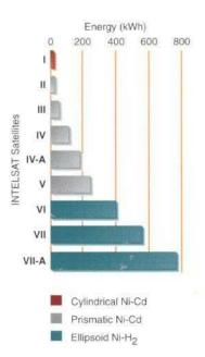
Battery capacity has increased significantly from generation to generation of communications satellites.
