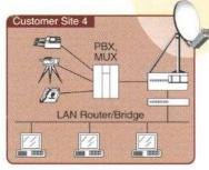
The BOD II system: Multiple transmission rates from 2 to 16 Mbit/s, adjustable on a burst-byburst basis, permit mesh connectivity for heterogeneous networks of both low-rate, low-cost customer premises terminals and higher-rate gateway hub terminals. FEC coding rates are also adjustable on a burst-by-burst basis, to permit integration of small and large earth stations into the network.
