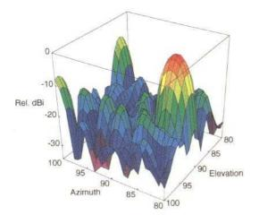
Testing of the Ku-band active phased array included measuring radiation patterns at multiple frequencies and power levels, performing holographic measurements, and evaluating system performance of intermodulation levels and bit error ratios under multicarrier conditions.
