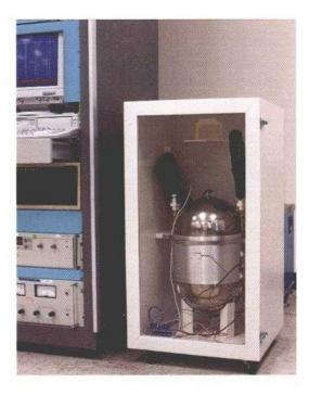
One of the new lightweight CPV batteries in SSTD's life test chamber.
