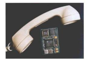
The COMSAT 1,200-bit/s LSF-Split VQ voice codec has been optimized to run on a miniature digital signal processing platform, enabling it to be used in a variety of voice telephony, digital radio, and voice messaging applications.
