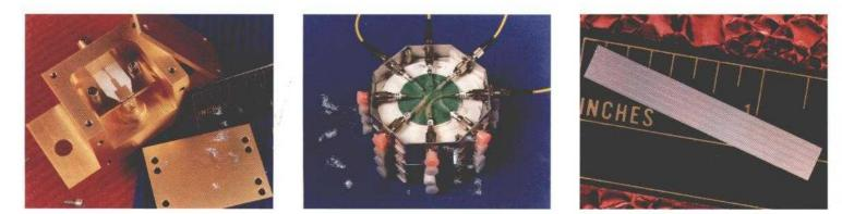
Three examples of optical technology ideally suited for satellite applications: LEFT: an impedance-matched high-efficiency microwaveoptical transmitter: CENTER: a true time-delay fiber optic beam-forming matrix for C-band phased-array antennas; RiGHT: an integrated optical waveguide and power splitter using state-of-the-art nonlinear materials. Each optical technology reduces onboard mass and power for lower satellite and launch vehicle costs.
