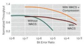
With the WACS, transmission control protocol/Internet protocol (TCP/IP) transfer performance is significantly improved.
