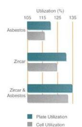
Destructive physical analysis of Ni-H<sub>2</sub> cells indicates that the coefficient of positive plate active material utilization is higher in cells containing two layers of Zircar<sup>1M</sup>, or one layer of Zircar<sup>1M</sup> and one layer of fuel-cell-grade ashestos, compared to cells with one layer of asbestos.
