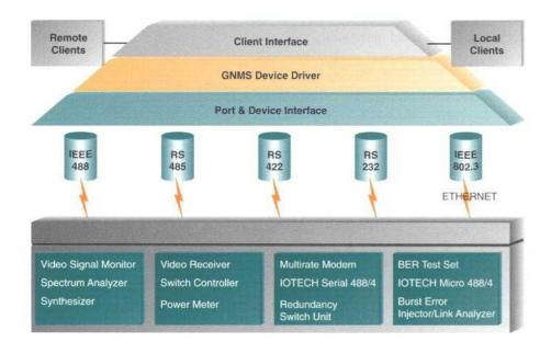
responses to the client applications. It sets up connections, monitors link status, and ensures that the device responses (or proper error returns) are returned to the clients in the correct sequence. The driver is designed so that multiple clients can simultaneously monitor and control devices, with the restriction that a single client application can control only one device at a time.
